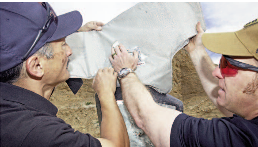
Even the .44 Magnum round fired from "the most powerful handgun in the world" could not penetrate the Alpha Elite's Level IIIA soft armor.
