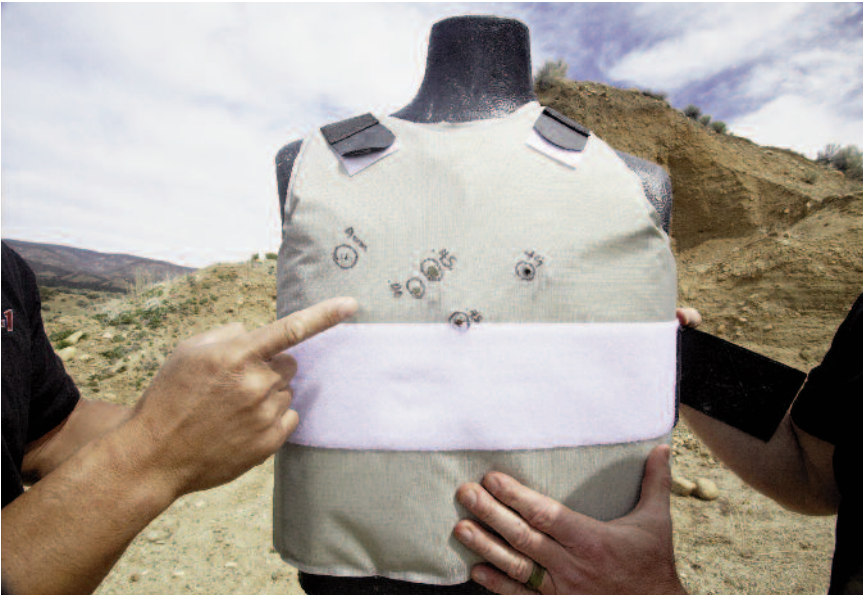
Each of the common pistol caliber tested fare against the Alpha Elite soft armor.
