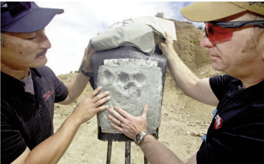
Chris Hirt of Point Blank Enterprise demonstrated that even blunt force trauma can be minimized using its tactical body armor due to its proprietary construction as shown by the clay indentation made by each of the pistol rounds.
