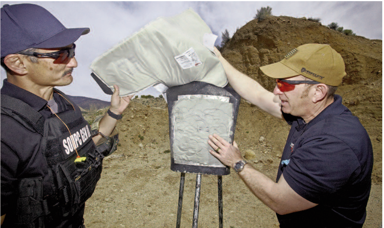
There was no damage to the back side of the SOST-500 armor plate. Even the potential trauma from the blunt force seemed minimal.
