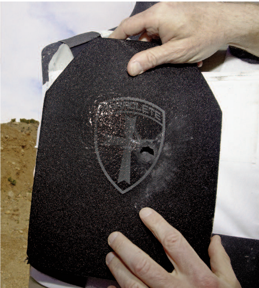
Removing the armor plate from the nylon cover revealed a gaping hole from a rifle round.
